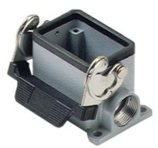
Surface mounting housing, C-TYPE series, with 1 lever, M40 x 2 cable entry, size "44.27", high construction
