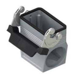
Hood, C-TYPE series, with 1 lever, M40 side cable entry without adapter, size "57.27", high construction
