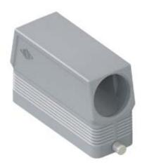
Hood, C-TYPE series, with 2 pegs, M32 side cable entry without adapter, size "104.27", high construction
