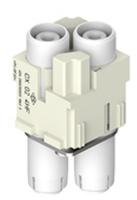
female modular insert, Mixo series, crimp connection, 2 poles, 2 modules, 40 A 2900/5000 V 15 kV 3, with heat-shrinking tube
