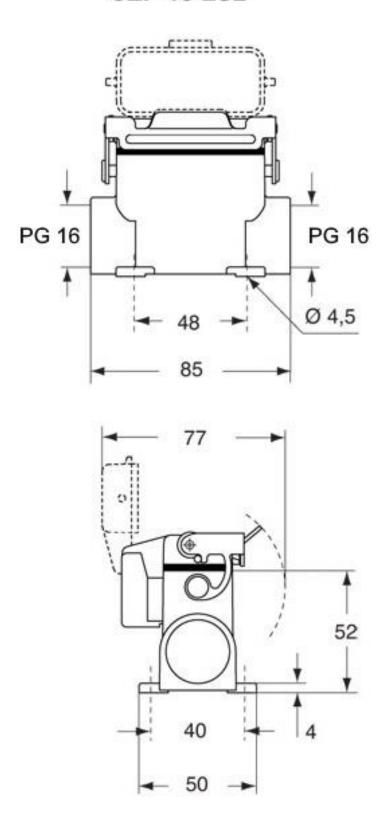
Dimensions in mm. Dimensions shown are not binding and may be changed without notice
