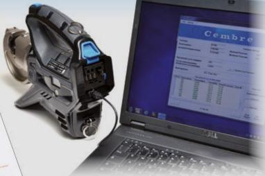
Pdf downloads summarise pressure & force validation data for the last 10 crimping cycles, while the .csv format downloads all data for up to 200,000 operating cycles.
